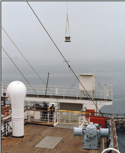
One of two 2.5-ton capstans is lifted by helicopter off the stern of Queen Mary, June 13, 1989.
